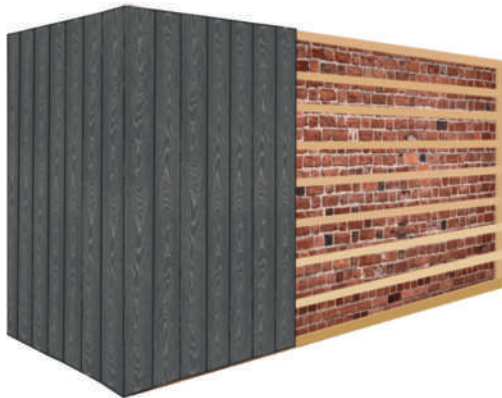
Vertical Board Horizontal Subframe
